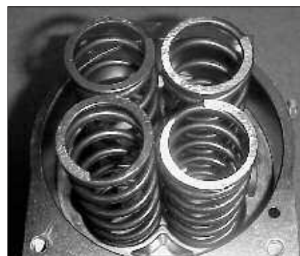
3. Locating of springs in piston head cavities
